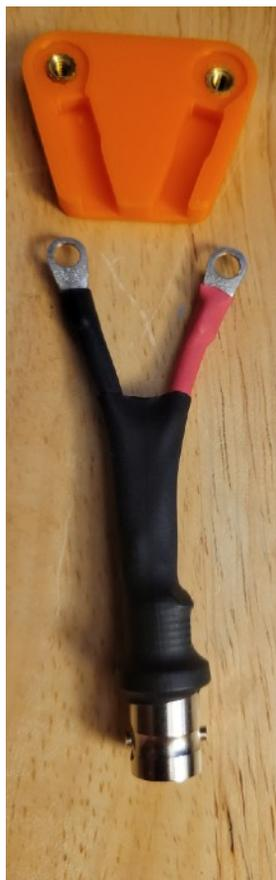
Attach 25 feet of RG-58 coax, and test by hanging the antenna.
