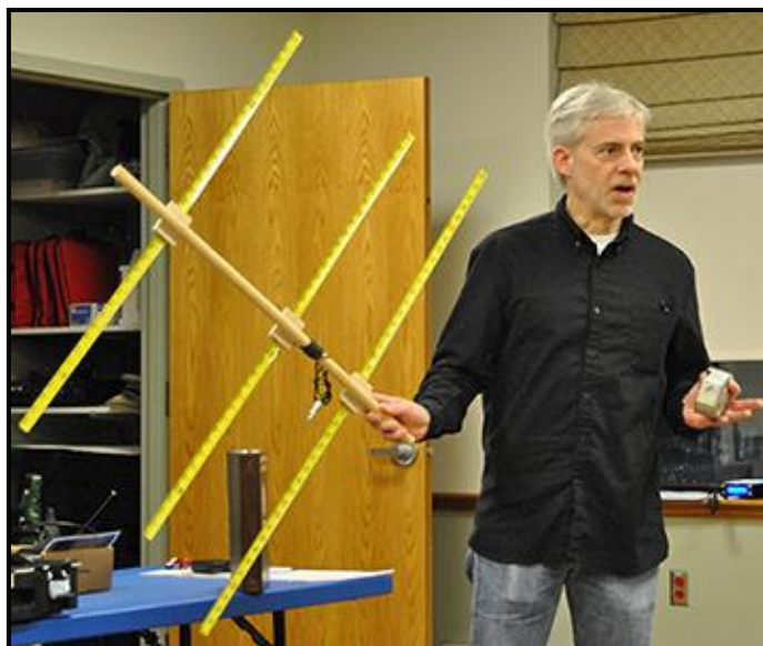
Alan, AB1XB, built a collapsible tape measure RDF yagi antenna. He'll be making a case for it next.
