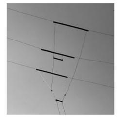
The terminated 3-Wire Folded Dipole (T3FD) is a very versatile multiband antenna.
